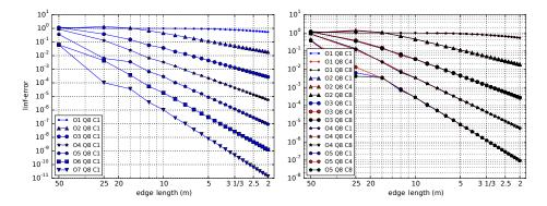
Fig. 2. Convergence of EDGE in the  $L^{\infty}$ -norm. Shown are orders  $\mathcal{O}1-\mathcal{O}7$  for the eighth quantity v (Q8) in non-fused runs on the left. The right plot shows orders  $\mathcal{O}1-\mathcal{O}5$  for v (Q8) when utilizing EDGE's fusion capabilities with shifted initial conditions. For clarity, from the total of eight fused simulations, only errors of the first (C1), fourth (C4) and last simulation (C8) are shown.
