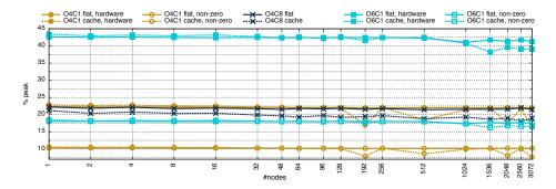
**Fig. 5.** Weak scaling study on Theta. Shown are hardware and non-zero hardware peak efficiencies of all configurations in cache and flat mode. O denotes the order and C the number of fused simulations.
