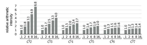
**Fig. 1.** Arithmetic intensity if the material parameters and mesh are shared in an elastic ADER-DG setup. Shown is the relative improvement over a non-fused simulation in dependency of the order  $(\mathcal{O}2-\mathcal{O}7)$  and the number of fused runs (1, 2, 4, 8, 16).
