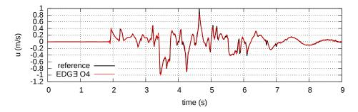
**Fig. 3.** Synthetic seismogram of EDGE for quantity u at the nith seismic receiver located at  $(8647 \,\mathrm{m}, 5764 \,\mathrm{m}, 0)$  in red. The reference solution is shown in black.
