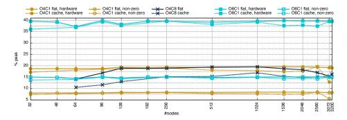
**Fig. 7.** Strong scaling study on Theta. Shown are hardware and non-zero peak efficiencies of all configurations in cache and flat mode. O denotes the order and C the number of fused simulations.
