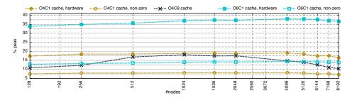
Fig. 8. Strong scaling study on Cori-II. Shown are hardware and non-zero hardware peak efficiencies of all configurations in cache mode. O denotes the order and C the number of fused simulations.
